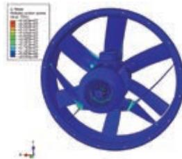
The cast aluminium's fatigue limit for 28.8 million cycles is about 80 MPa. All Aluminium parts have a stress below 65 MPa, so all this parts meet the requirements. The steel's fatigue limit is much higher than aluminium, so all steel parts meets too the requirements.
