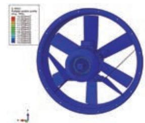
The test result confirms that the fan can resist the impact required by the standard, because 23.5 MPa is a stress value too low for steels.
