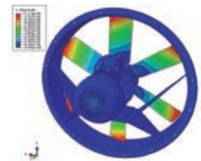
Fan's stress map after the impact. The maximum stress is 23.5 MPa for all axes; it is situated in the steel frame.
