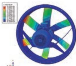
Fan's stress map after the test. The maximum stress is 69.7 MPa for steel parts and 65 MPa for aluminium parts. It is the maximum for all axes.
